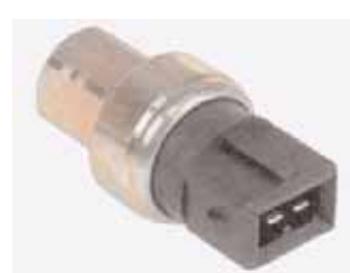
MC-1305 Volvo Cycling Switch - Female M12-1.5 Thd. Open 24 PSI - Close 44 PSI (NO) 94 - 97 Volvo (Replaces MT0210)
