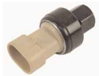
MC-1319 Peterbilt High Pressure Switch Female M10-1.25 Open 200 PSI - Close 270 PSI (NO) OEM #18-03836, P93CAA3606-1
