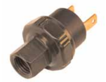
MC-1313 Binary Switch Female 7/16-20 Thd. 27 PSI - 170 PSI
