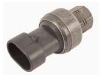
MC-1320 Peterbilt High Pressure Switch Female M10-1.25 Open 330-370 PSI - Close 180-240 PSI (NC) OEM #18-03835, P93CAA3605-1
