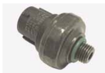
MC-1279 Binary Switch - Male 3/8-24 Thd. Open 375 PSI - Close 451 PSI - Open 28 PSI (NC) 90-93 Acura / Honda, 98 - 99 Isuzu (Replaces MT0397)
