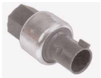
MC-1306 GM Cycling Switch - Female M12- 1.5 Thd. Open 24 PSI - Close 44 PSI (NO) 90 - 96 Cars, 94 - 00 Trucks (Replaces MT0205)
