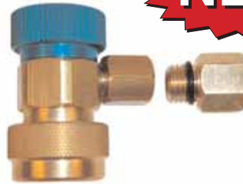
TL5109 HFO-1234yf Low Side Charging Coupler Includes Low Side Quick Connect Coupler with (1) MC-1343 Metric Threaded Adapter for R-134a Charging Hoses
